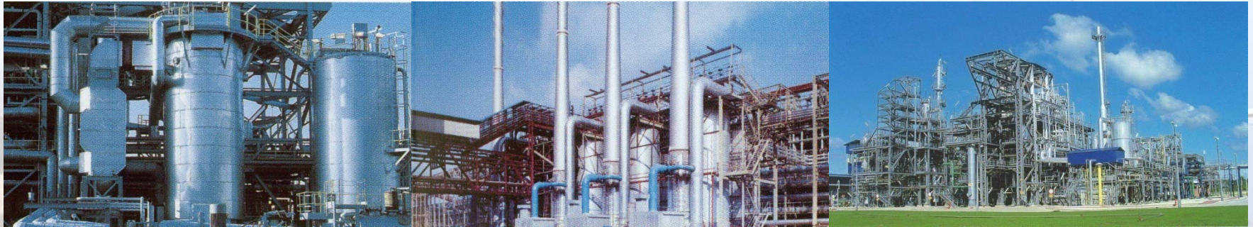
a) Molten Salt system with an output of 14 MW at 430° C, England
