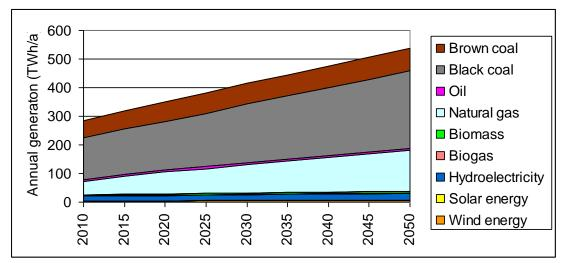
**Figure 1**: Option 1 – Business as Usual, annual electricity generation (TWh/a). Projections to 2030 from ABARE (2007). The trends from 2020 to 2030 were extended to 2050. The technologies in this chart are the technologies in the ABARE projections. In the charts in the following sections the bottom seven technologies in the chart legend, and the energy they supply, are identical for all options.
