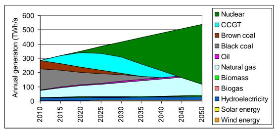
**Figure 3**: Option 3 – Nuclear and CCGT, annual electricity generation (TWh/a). The seven technologies listed at the bottom of the legend supply the same amount of energy in all six options. Black coal and brown coal supply the same energy in all options except the Business as Usual option. The technologies listed above Brown coal in the legend are the replacement for the decommissioned coal generators.
