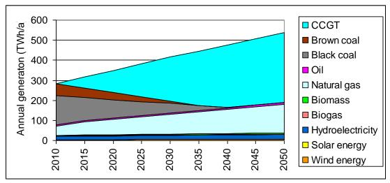
**Figure 2**: Option 2 - CCGT, annual electricity generation (TWh/a). The seven technologies listed at the bottom of the legend supply the same amount of energy in all options <sup>13</sup>. Black coal and brown coal supply the same energy in all options other than the Business as Usual option. The technologies listed above Brown Coal in the legend are the replacements for the decommissioned coal generators.
