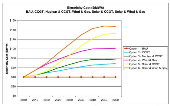
Figure 10: Electricity cost for the six options. (\$/MWh sent out, Constant 2009 \$)
