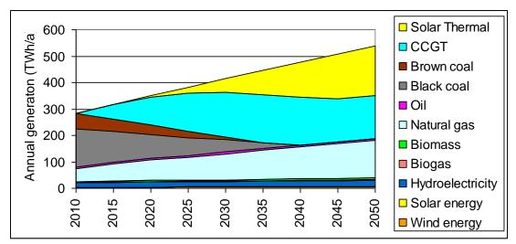
**Figure 5**: Option 5 – Solar thermal and CCGT annual electricity generation (TWh/a). The seven technologies listed at the bottom of the legend supply the same amount of energy in all six options. Black coal and brown coal supply the same energy in all options except the Business as Usual option. The technologies listed above Brown coal in the legend are the replacement for the decommissioned coal generators.
