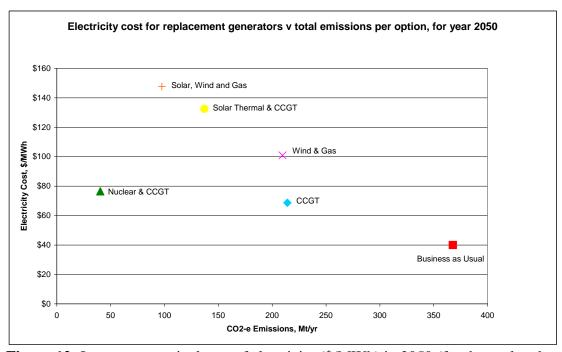
**Figure 12:** Long run marginal cost of electricity (\$/MWh) in 2050 (for the coal and replacement technologies only) versus total emissions (t CO2-e/MWh) from all the technologies in each option.
