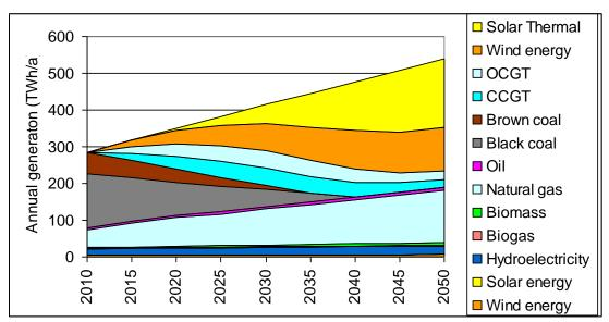
**Figure 6**: Option 6 – Solar thermal, wind and gas; annual electricity generation (TWh/a). The seven technologies listed at the bottom of the legend supply the same amount of energy in all options. Black coal and brown coal supply the same energy in all options other than the Business as Usual option. The technologies listed above Brown Coal are the replacements for the decommissioned coal generators.
