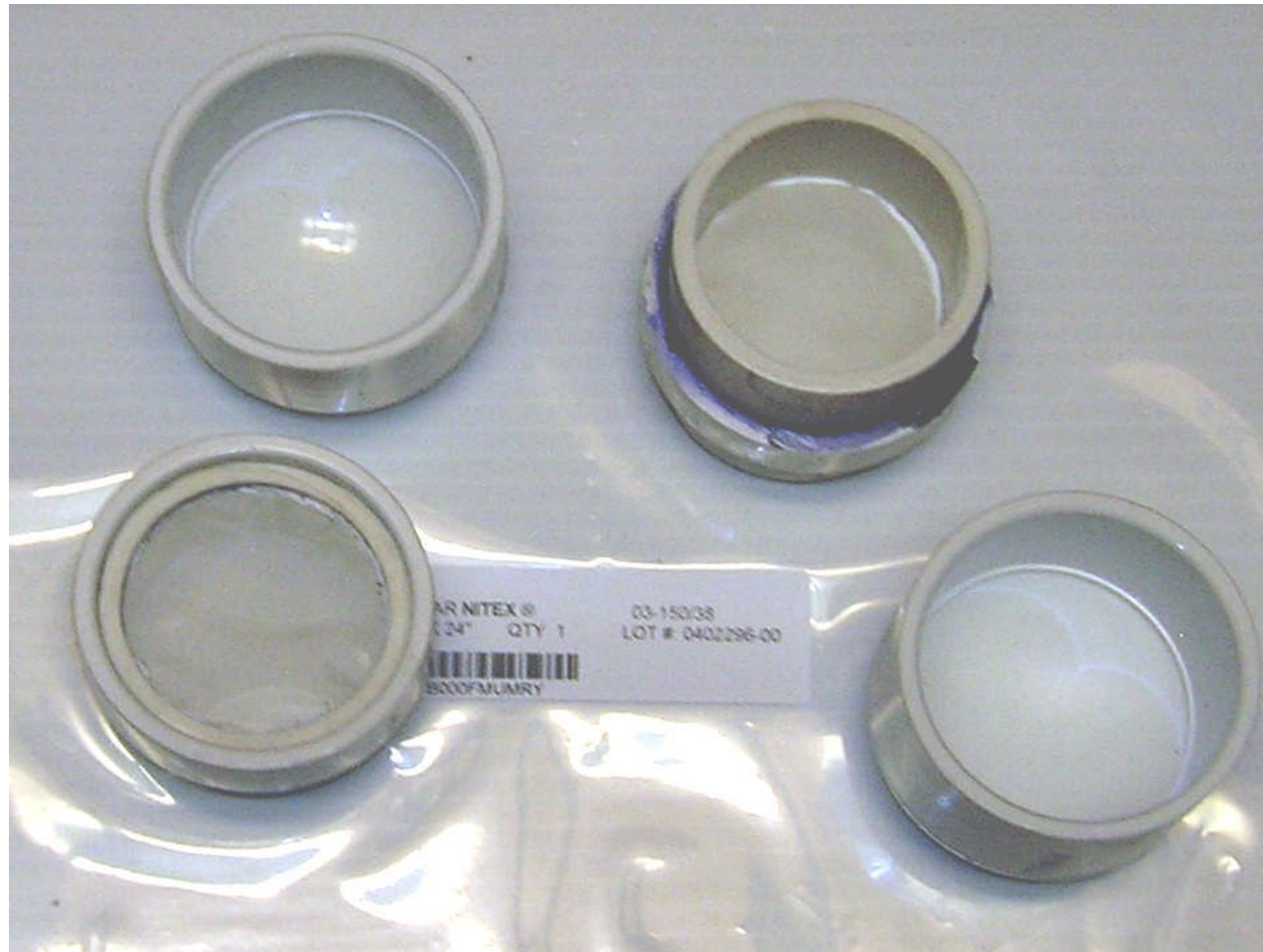
PCT sample screens: 150 & 75 \mu NITEX™, silicone glue, & 2" PVC pipe fittings
