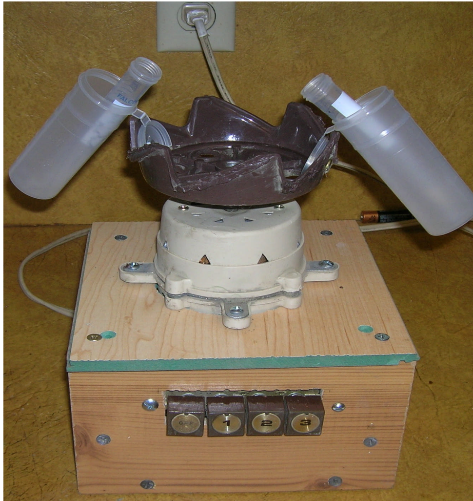
CENTRIFUGE: 3 speed fan, faux wood flooring, plastic snap vials, barbell plate, screws, etc.
