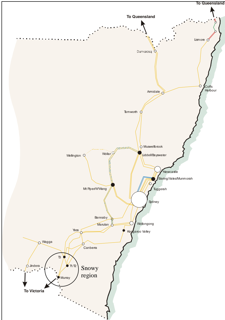
Figure 2.3: Main NSW and Snowy Transmission System
