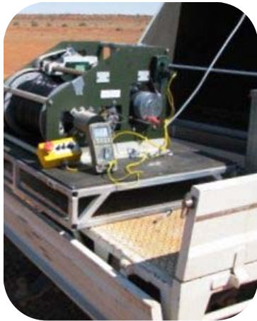
Torrens Energy Vehicle mounted temperature logging equipment.
