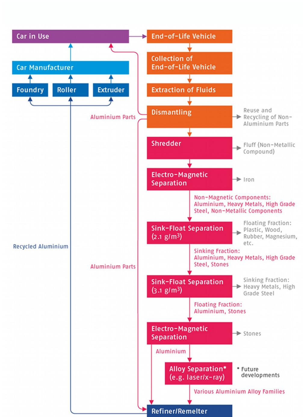
**Figure 10: Modern End-of-Life Vehicle Dismantling and Aluminium Recycling Process**
