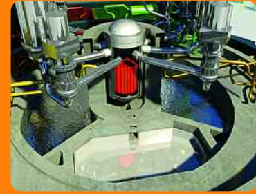
The core melt retention system provides corium confinement inside the reactor building.
