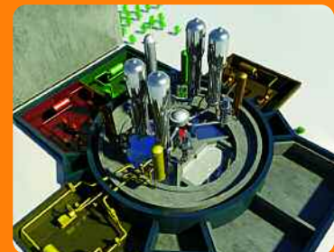
One train of each safeguard system in each of the four safeguard building, the core catcher and the in-containment refueling water storage tank.
