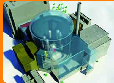
The double-concrete shell covers the nuclear system, the fuel building and two of the four safeguard buildings.
