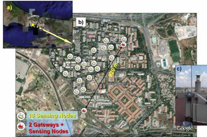
Fig. 23 SOSEWIN prototype installation in Istanbul. In the district east of the international airport of Istanbul 20 SNs are installed, two of them are connected to the Internet with DSL lines. This internet connection is used to data transfer for the involved partner institutes in Turkey and Germany.
