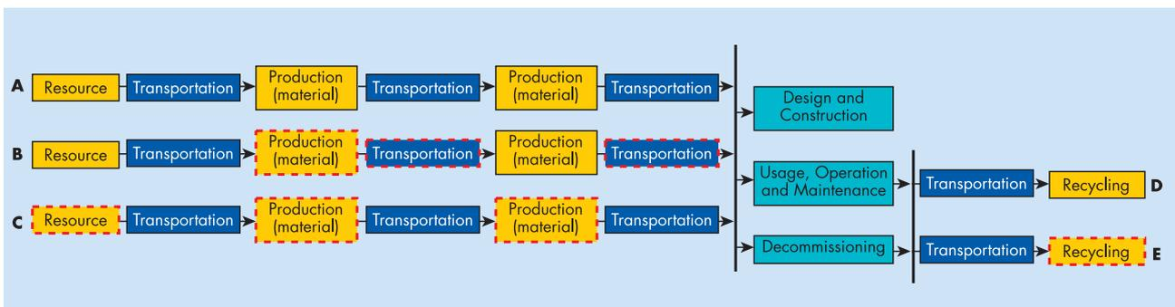
Typical process tree regarding construction and operation of nuclear power plants as well as examples of materials from each branch:
