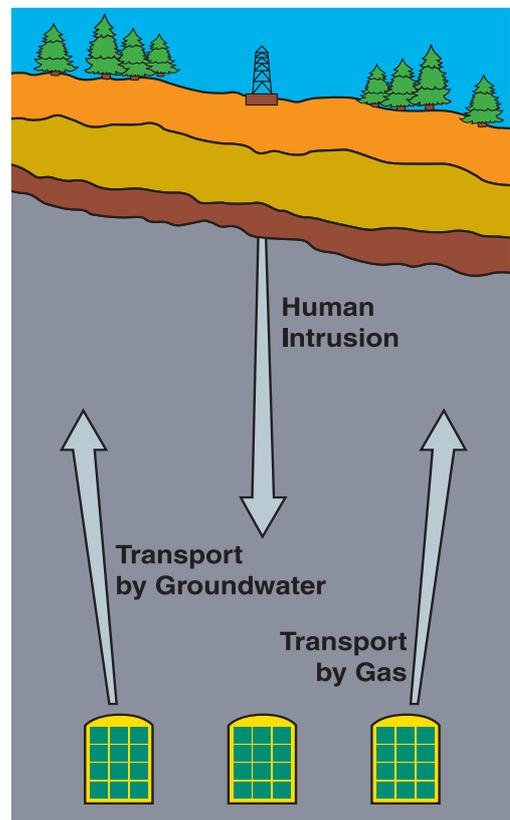
Figure 13. Schematic illustration of main assessment pathways (not to scale)
