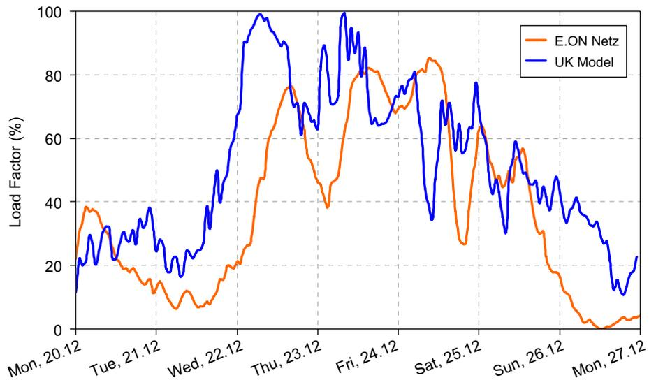
Fig. 10. Actual wind load factors in the E.ON Netz control area, and UK wind power model, 20–26 December 2004.
