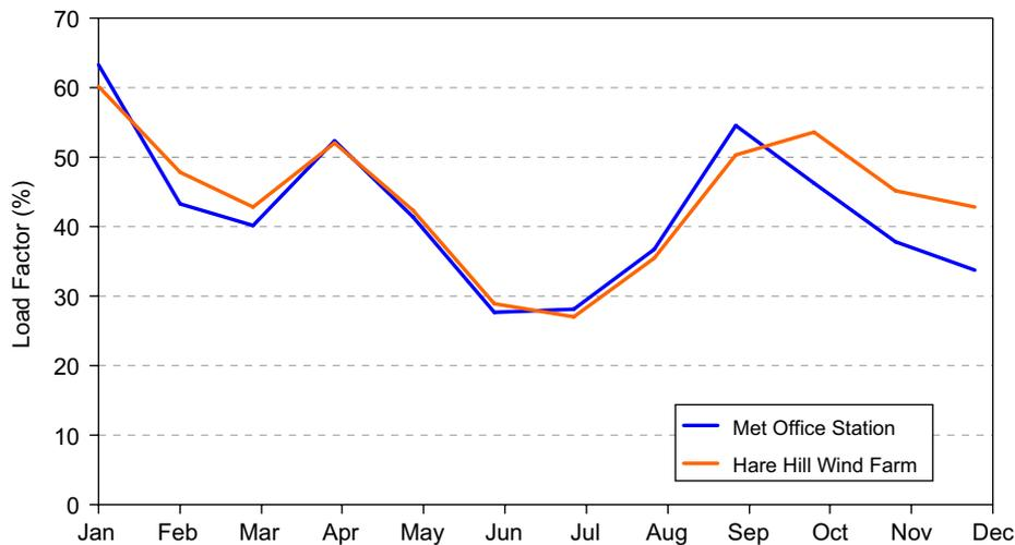
Fig. 5. Calibrated theoretical power and actual output for the Hare Hill Wind Farm in Cumbria. Scale factor used = 1.2.
