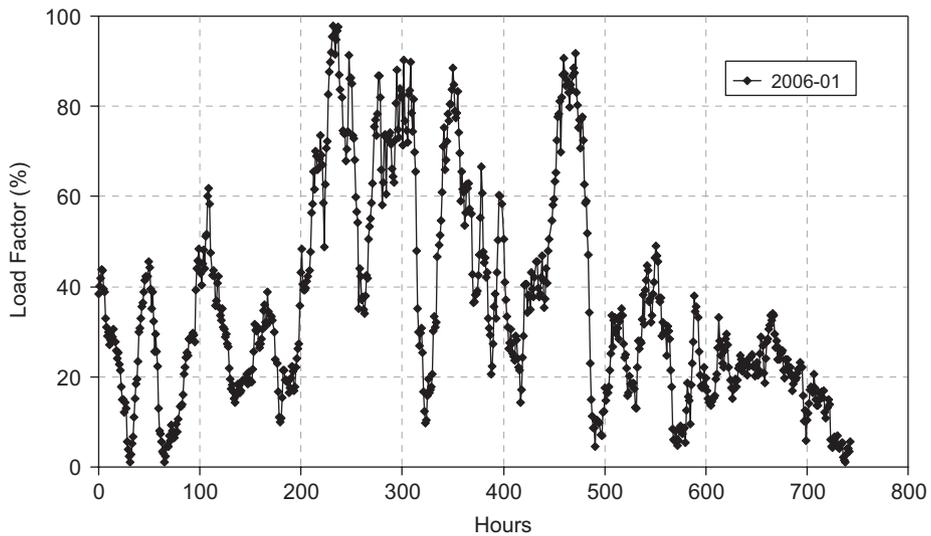
Fig. 7. Modelled aggregate power for 25 GW of wind, January 2006.
