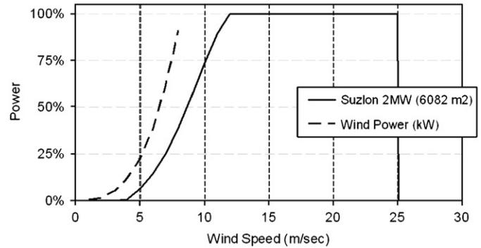
Fig. 3. Wind turbine power curve.
