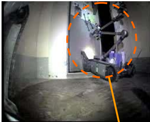
Opening a double door (April 18)
