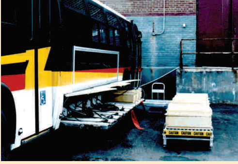
Refueled Zinc-Air fuel cell modules ready for installation on bus
