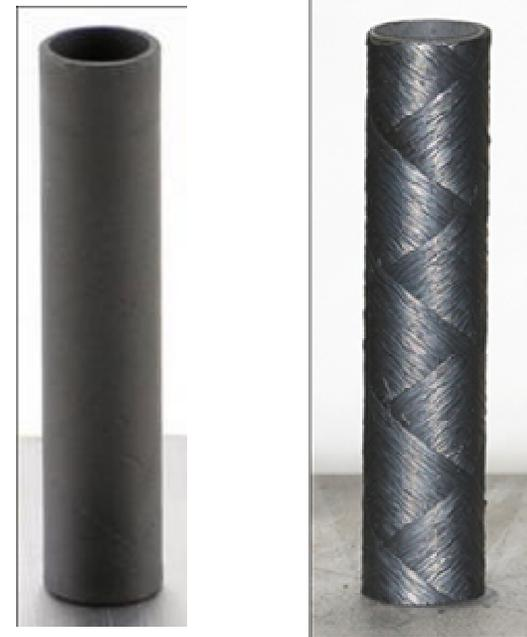
Triplex SiC cladding tube (monolith, fiber composite, and barrier coating are all SiC)
