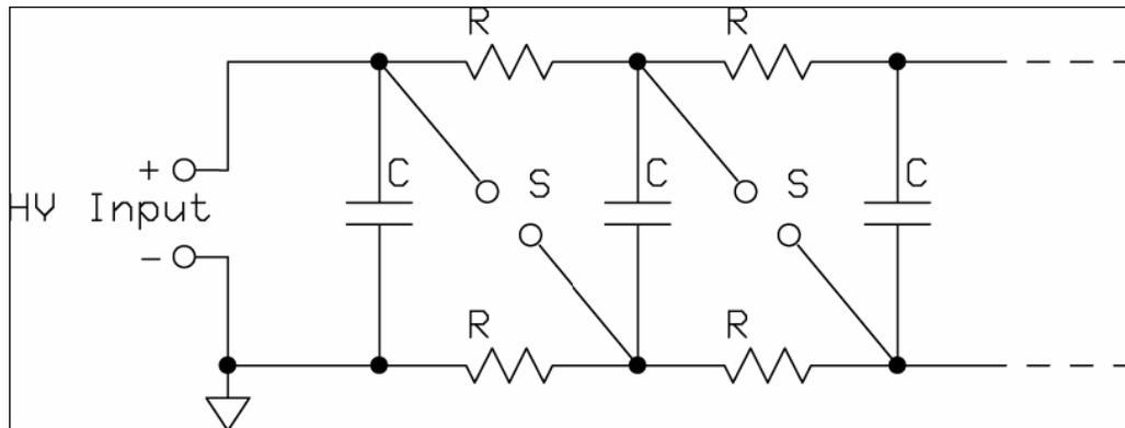
**Figure 7:** In an “ordinary” Marx generator  $n$  capacitors  $C$  charged up to the voltage  $v$ , and are over spark gaps switched into series, adding up their voltages to the voltage  $V = nv$ .
