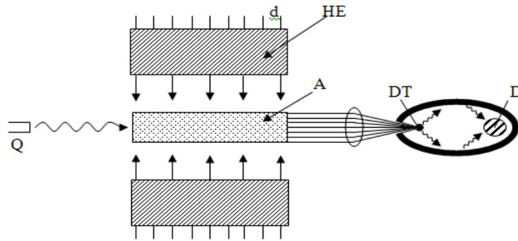
**Figure 5** Argon ion laser igniter, to ignite a staged DT  $\rightarrow$ DD fusion explosion in a mini-Teller-Ulam configuration. **A** solid argon rod. **HE** cylindrical shell of high explosive, **d** detonators. **Q** Q-switched argon ion laser oscillator.
