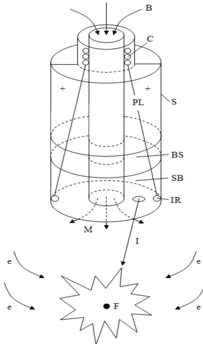
**Figure 4** Superconducting “atomic” spaceship, positively charged to GeV potential, with azimuthal currents and magnetic mirror **M** by magnetic field **B**. **F** fusion minibomb in position to be ignited by intense ion beam **I**, **SB** storage space for the bombs, **BS** bioshield for the payload **PL**, **C** coils pulsed by current drawn from induction ring **IR**. **e** electron flow neutralizing space charge of the fusion explosion plasma.
