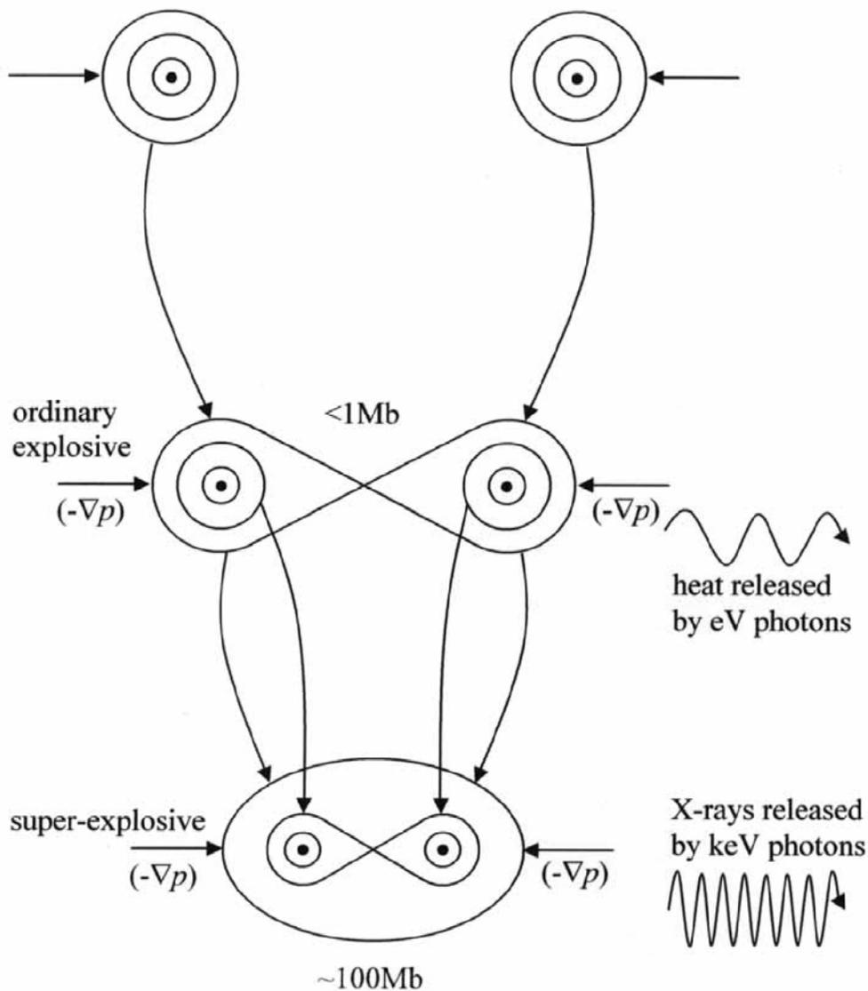
**Fig.A1** In an ordinary explosive the outer shell electrons of the reacting atoms form “eV” molecules accompanied by the release of heat through eV photons. In a superexplosive the outer shell electrons “melt” into a common outer shell with inner electron shells form “keV” molecules accompanied by the release of X-ray keV photons.
