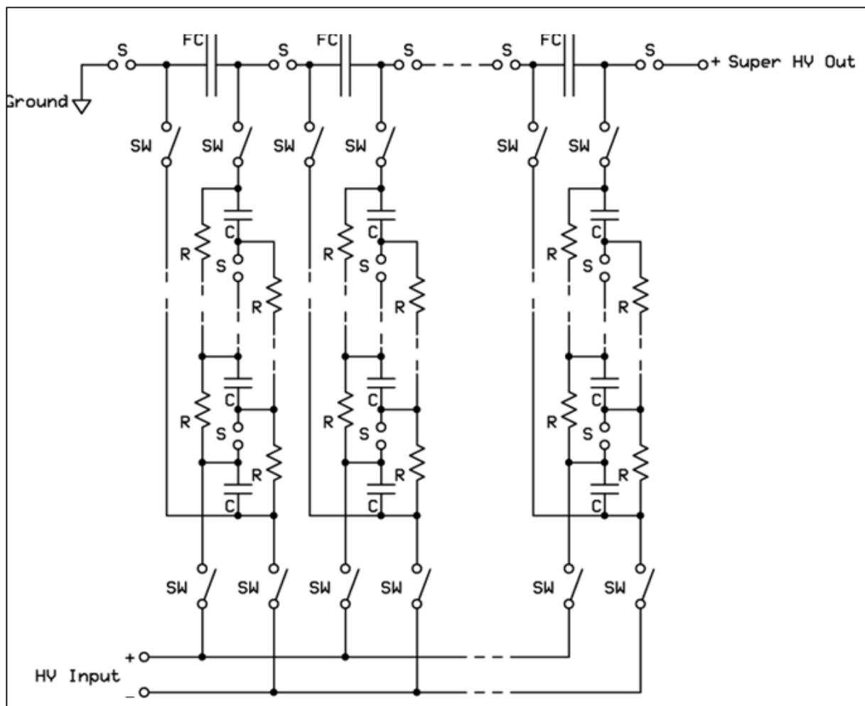
**Figure 8:** In a Super Marx generator,  $N$  Marx generators charge up  $N$  fast capacitors  $FC$  to the voltage  $V$ , which switched into series add up their voltages to the voltage  $NV$ .
