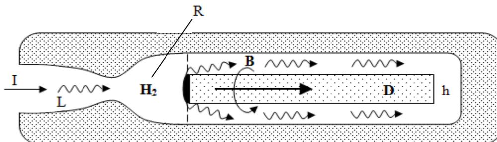
**Figure 2** Pure deuterium fusion explosion ignited with an intense ion beam. **D** deuterium rod, **h** hohlraum, **I** ion beam, **B** magnetic field, **R** miniature target rocket chamber, **H<sub>2</sub>** solid hydrogen, **L** laser beam to heat hydrogen in miniature rocket chamber.
