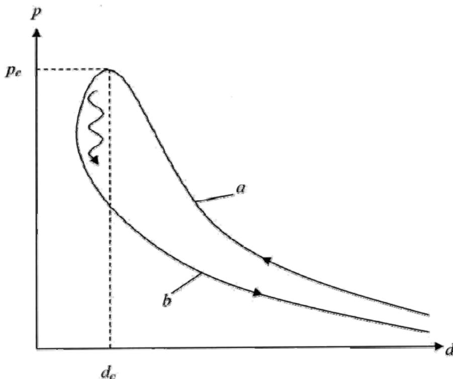
**Fig. A3.**  $p$ - $d$ , pressure – inneratomic distance diagram for the upper atomic and lower molecular adiabat.
