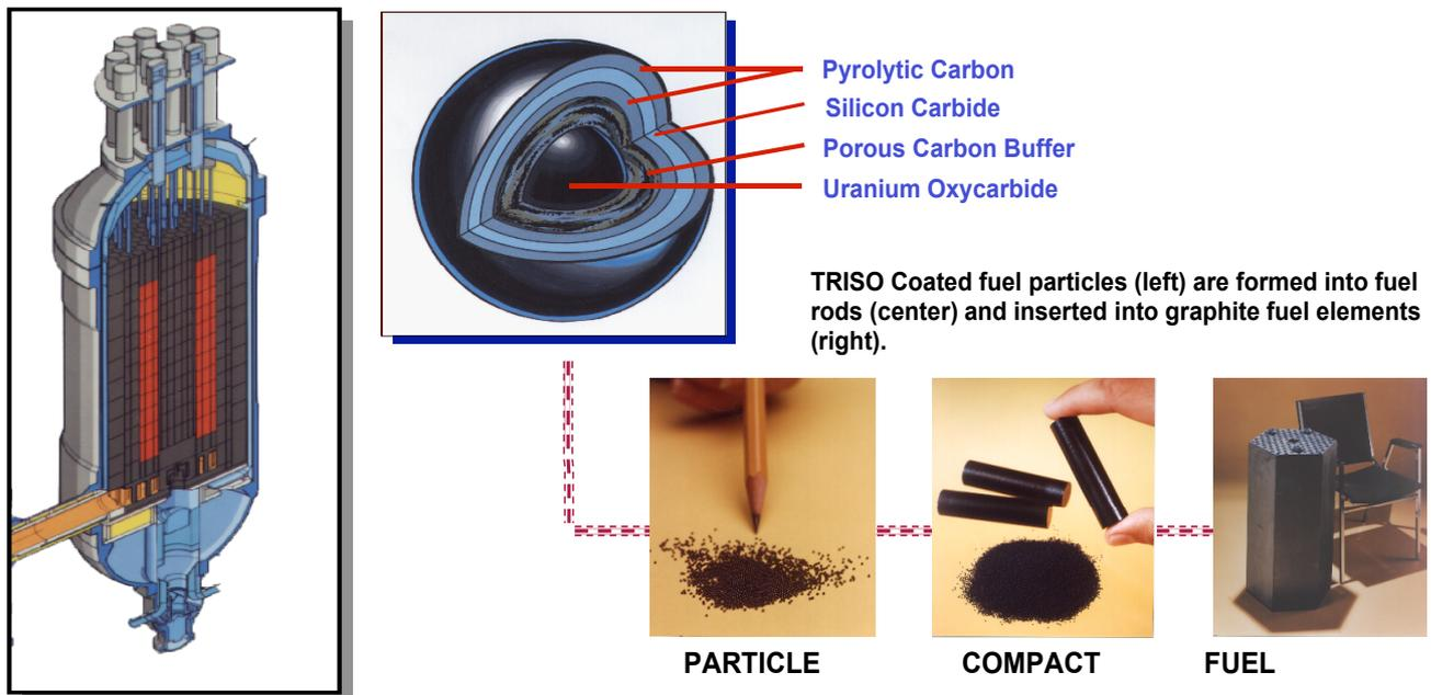
**Figure 7: Conceptual Picture of MHGR and TRISO Fuel for Prismatic Core and PBMR Fuel**
