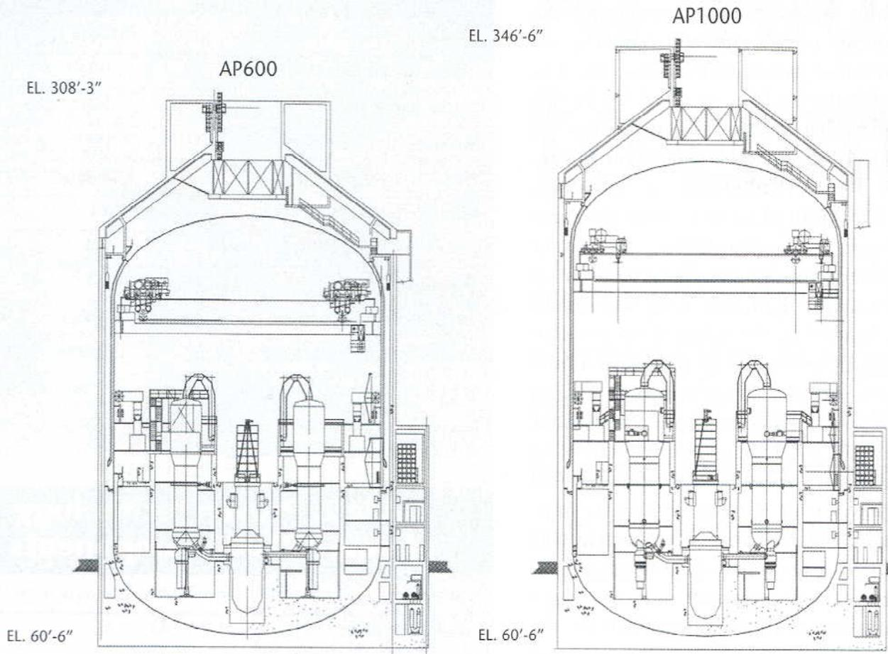
**Figure 4: AP600 & AP1000 Comparison and Overall Plant Conceptual Figure**
