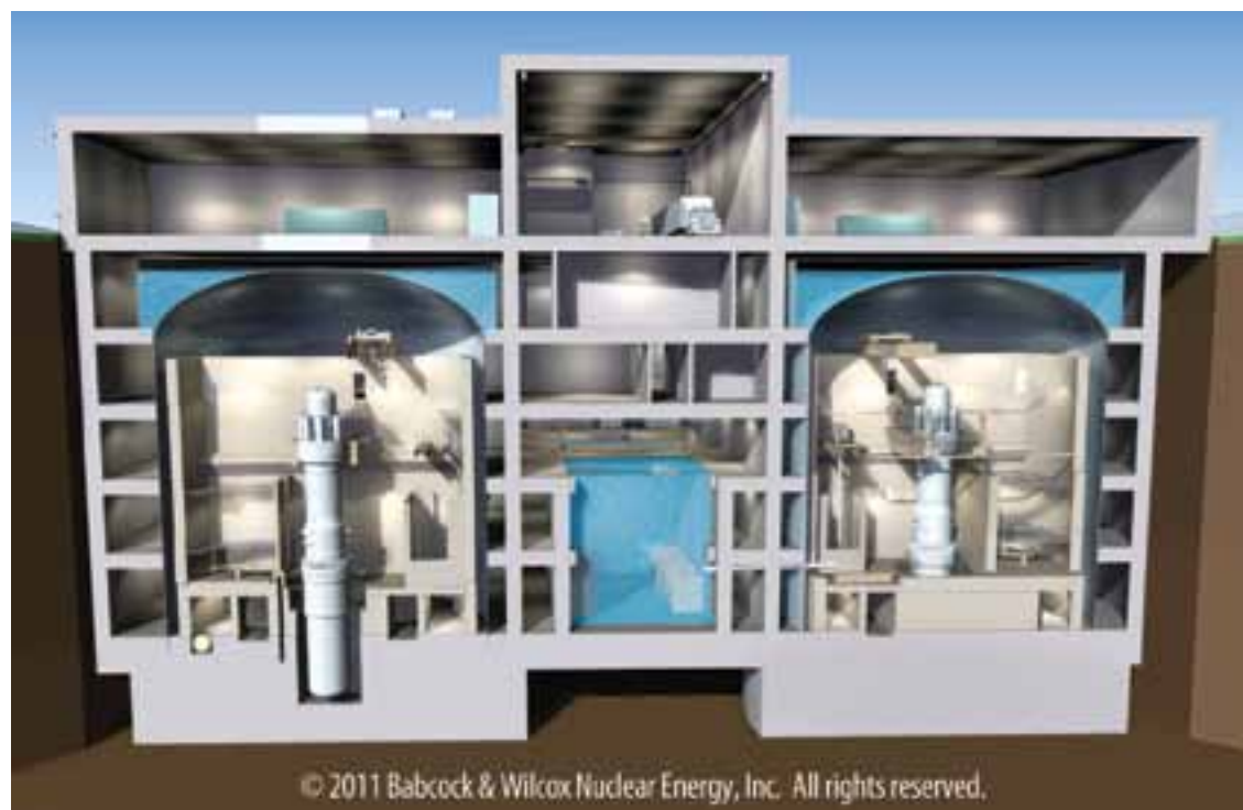
Conceptual drawing of a two module reactor, featuring full underground reactor containment, reservoirs for emergency passive cooling (top left and right) and fully contained below-ground spent fuel cooling pond (bottom centre).
