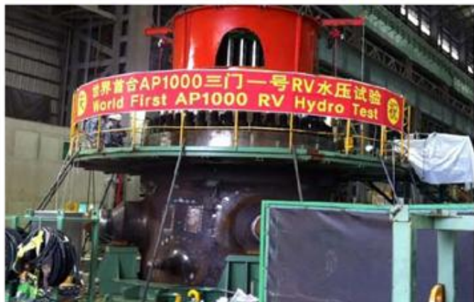
Finished hydro test
