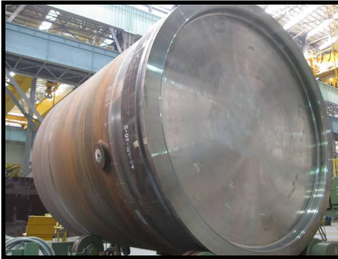
SG Lower Shell and Tubesheet – Unit 2B
