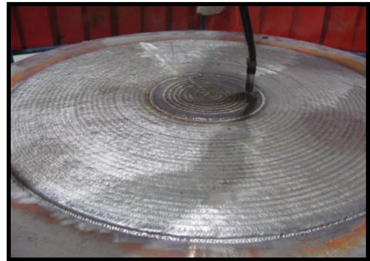
Cladding Techniques – Robot Welder
