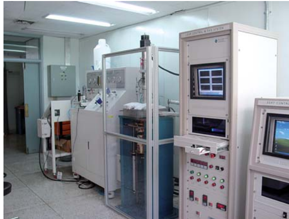
Figure 4.8 - Corrosion and SCC Test Loop
