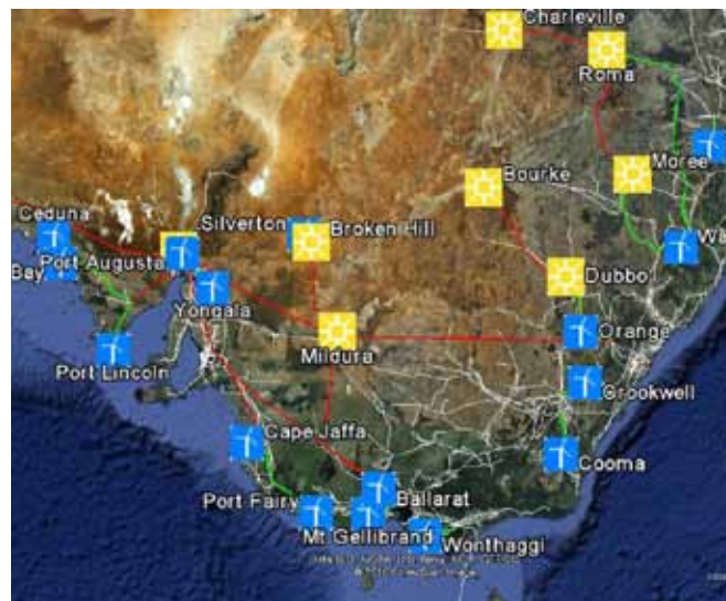
Figure 5 and 6: ZCA2020 Overview Map. Yellow squares represent solar thermal sites, and blue squares represent wind sites. Red lines represent new HVDC transmission lines and green lines represent new HVAC transmissions lines.
