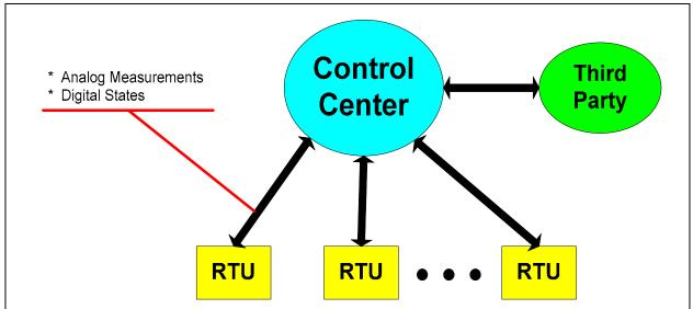
Figure 1: The Control Center has direct communication channels to the Remote Terminal Units (RTU) at each Substation and Generating Station
