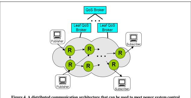
Figure 4. A distributed communication architecture that can be used to meet power system control requirements of the future.
