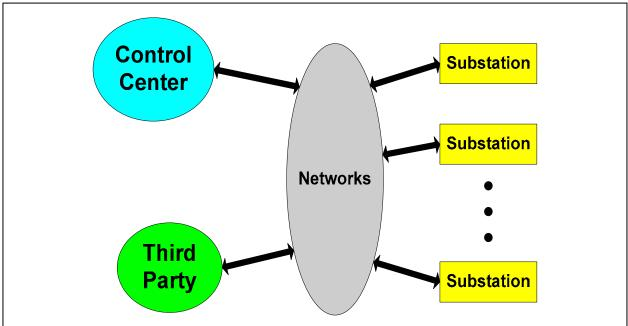
Figure 3. In time the communication channels between substations and control center will be replaced with a high bandwidth dedicated network that will allow faster area-wide controls.
