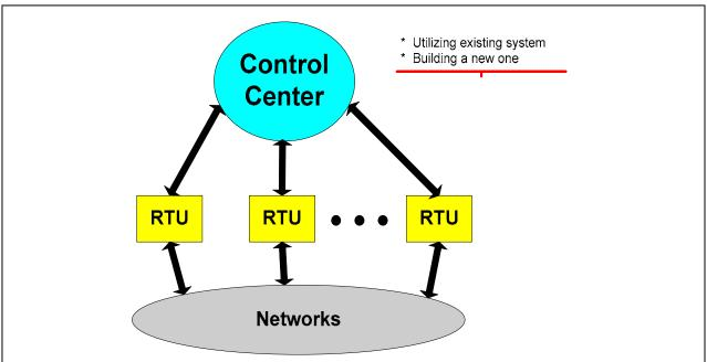
Figure 2. Substations today are measuring more real time data than can be sent over the communication channel capacities to the control center. However, stored data can be moved slowly over other computer networks.
