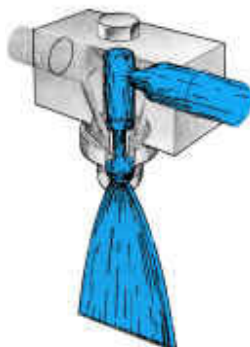
Figure 25: Twin Fluid Atomization Nozzle with Flat Fan Spray Pattern (TPS, Inc., 1999)
