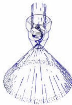
Figure 23: Hollow Cone Nozzle and Spray (TPS, Inc., 1999)
