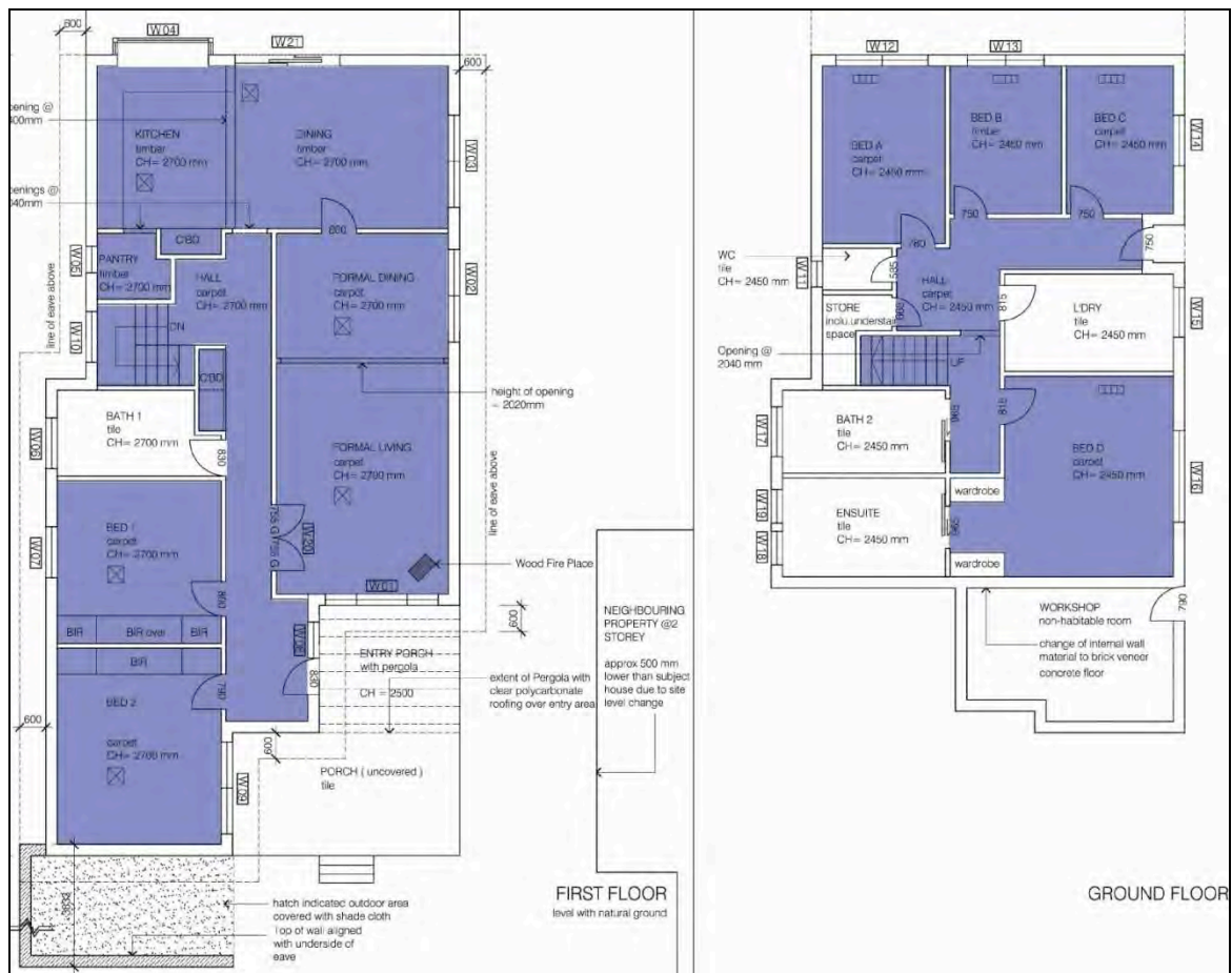
Figure 2: Conditioned zones in energy rating mode and actual conditioning mode
