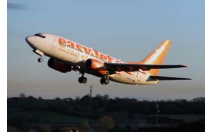
Figure C.11. Boeing 737-700: 30 kWh per 100 passenger-km. Photograph © Tom Collins.
