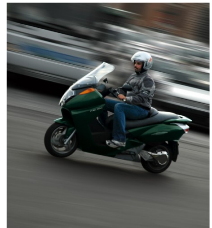
Figure 20.44. Vectrix: 2.75 kWh per 100 km . Photo from www.vectrix.com .
