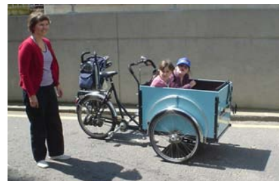
Figure 20.3. “Babies on board.” This mode of transportation has an energy cost of 1 kWh per 100 person-km.
