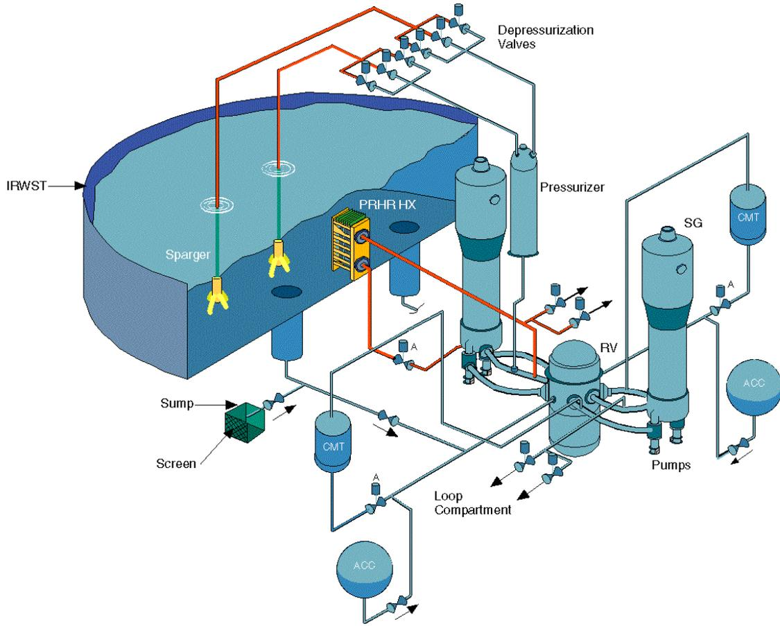
**Figure 4 – AP1000 RCS and Passive Core Cooling System**
