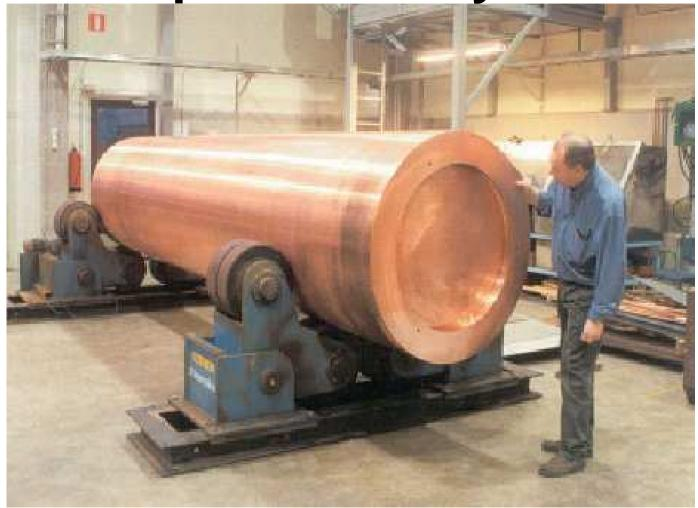
Example of a wasteform: copper canister for deep disposal of spent nuclear fuel in Sweden and Finland
