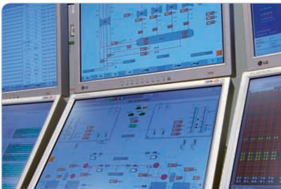
Turbine control displays. Using the simulator, operators can practise controlling the power plant without interfering with its actual normal operations.
