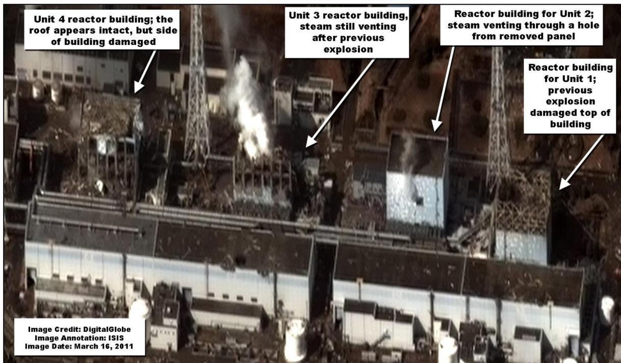
Figure 5. Satellite image taken at 9:35am on March 16. Plumes can be seen venting out of reactor buildings 2 and 3.
