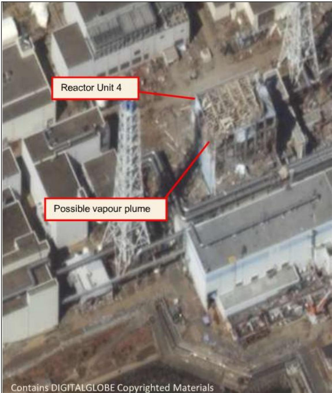
*Figure 10. A satellite image taken on 10:19am on March 18th from an IAEA presentation. The IAEA observes a “possible vapor plume” on the southeast corner of the unit 4 building.*
